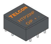
The HTP25NP is a closed loop Hall Effect Current Transformer suitable for measuring currents up to 25A. The product provides an output current, galvanically isolated from the primary conductor into an external load resistance. All contacts, including the primary are designed for PCB mounting.
